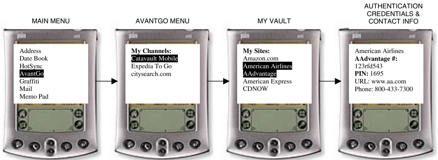
Figure 14: PDA Synchronization Functionality with AvantGo – Flow Chart
